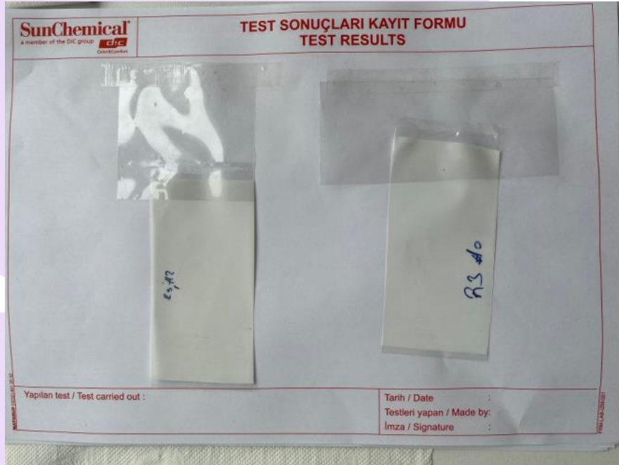
Figure 3: #0 and #2 bar results of tetrahydrofuran application of R3 ink formulation
